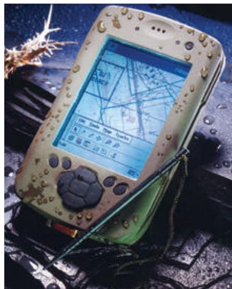
RPDA-88 is produced in four models, the smallest of which weighs less than 380 gm. Its touch-sensitive color-reflective display, built-in loudspeaker and
