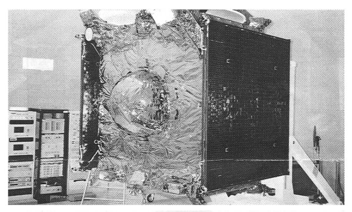
The rectangular shaped Amos is built around a circular cylinder which contains two propellant tanks, one for fuel and the other for oxidizer.
