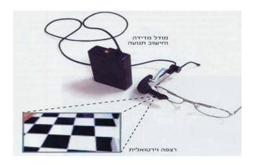
chessboard." Using an artificial nerve network, the device learns the patient's characteristic behavior and adapts the system's reactions to it.
