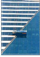
The first SkyBot can be seen by Tel-Avivians as it cleans the exterior of one of the city's burgeoning skyscrapers. The robot is claimed to work 30 times faster, if the same job is carried out manually. It is said to reduce the cost of cleaning by 90%.
